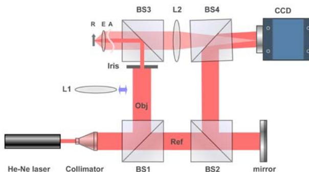
Fig. 1 Schematic of the Fourier Transform digital holographic adaptive optics imaging system. R:Retina, E:eye lens of focal length 25mm, A:aberrator. L1:75mm in focal length. L2:200mm. BS1-4: beamsplitters.
