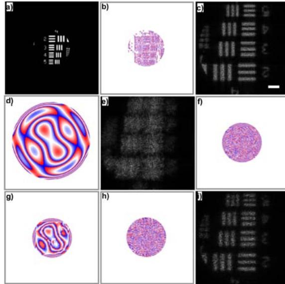
Fig.2 Simulations. a) and b) : simulated amplitude and phase. c): image without aberrator in place. d): simulated phase aberration. e): distorted image. f): the phase map of distorted field at the eye pupil. g):the measured phase aberration at the eye pupil. h): the phase map of the corrected field at pupil. i): the corrected image. scale bar: 100 $\mu$ m.
